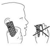
communication quality, may cause the device to operate at a higher power level than otherwise needed and may reduce the battery life.
