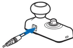
3. When the battery is fully charged, the red indicator light turns off. Disconnect the charger from the headset and the wall outlet.
