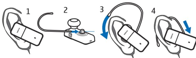
To use the headset on the left ear, rotate the earloop so that the loop is to the left of the text (5).
