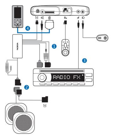
Disconnect the two ISO connectors from the car radio for power and loudspeakers, and replace them with the two connectors of the system cable CA-139.
