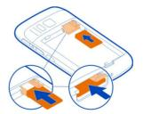
6 Line up the battery contacts, and insert the battery.
