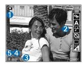
self-timer or sequence mode, or select the exposure compensation, white balance, and color tone (the active toolbar is not displayed during image capture). See "Active toolbar", p. 16.
