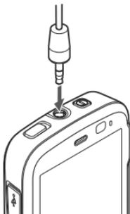
You can also connect a compatible TV-out cable to the Nokia AV Connector (3.5 mm) of your device.
