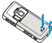
**2** To release the (U)SIM card holder, slide the holder to the right, and lift the holder up.
