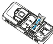
**3** Insert the (U)SIM card into the card holder. Ensure that the bevelled corner on the card is facing the bevelled corner on the holder, and that the contact area on the card is facing down. Slide the holder to the left, back to the slot to lock the holder into place.
