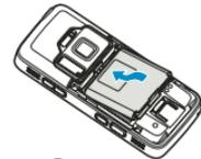
**5** Replace the cover so that the locking catches are directed towards their slots, and slide the cover into place.
