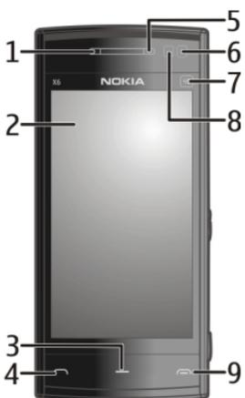
A grayscale diagram of a Nokia mobile phone. The phone is oriented vertically. At the top, there is a speaker grille (1) and a secondary camera lens (6). Below the camera is a proximity sensor (8). The main screen is a large touch screen (2). At the bottom of the phone, there is a navigation pad (3) with a central call button (4) and a power button (9). The Nokia logo and the number '16' are visible above the screen. |
