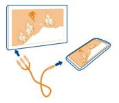
Do not connect products that create an output signal, as this may damage the device. Do not connect any voltage source to the Nokia AV connector. If you connect an external device or headset, other than those approved by Nokia for use with this device, to the Nokia AV connector, pay special attention to volume levels.
