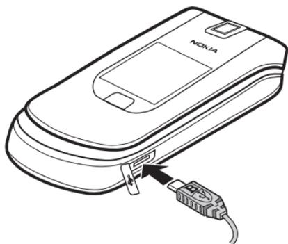
You may also charge the battery using a USB data cable with power from a computer.
