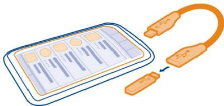
The Files application opens, and the memory stick is displayed as a mass memory
