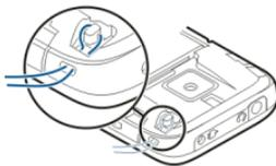
Thread the wrist strap as shown, and tighten it.
