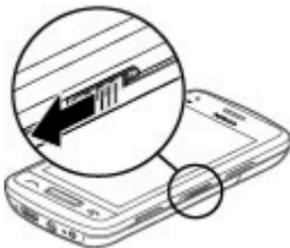
**Tip:** If the key lock switch is out of reach, to unlock the device, press the menu key, and select **Unlock**.
