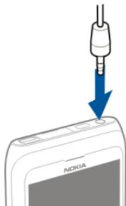
Do not connect products that create an output signal, as this may damage the device. Do not connect any voltage source to the Nokia AV connector. If you connect an external device or headset, other than those approved by Nokia for use with this device, to the Nokia AV connector, pay special attention to volume levels.
