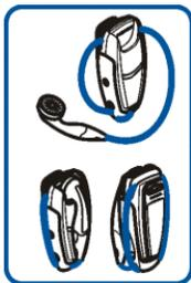
When you don't use the headset, you can wind the earphone wire around the headset as shown in Figure 6.
