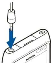
Do not connect products that create an output signal, as this may damage the device. Do not connect any voltage source to the Nokia AV connector. If you connect an external device or headset, other than those approved by Nokia for use with this device, to the Nokia AV connector, pay special attention to volume levels.
