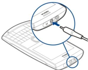
Do not connect products that create an output signal, as this may damage the device. Do not connect any voltage source to the Nokia AV connector. If you connect an external device or headset, other than those approved by Nokia for use with this device, to the Nokia AV connector, pay special attention to volume levels.
