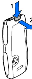
2. Remove the battery by lifting it as shown. Insert the SIM card into the SIM card holder until it snaps into position. Make sure that the SIM card is properly inserted and that the golden contact area on the card is facing downwards.
