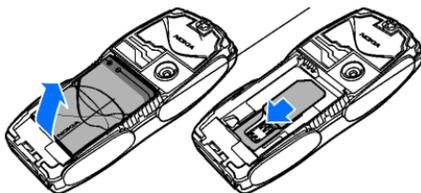
3. To remove the SIM card press the card release (1) and slide the SIM card towards the top of the phone (2).
