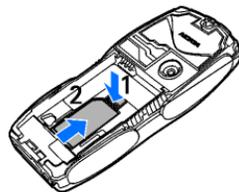
4. Replace the battery. Observe the contacts of the battery
