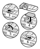
3 Line up the battery contacts, and insert the battery. Replace the back cover.
