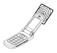
The reading range is typically 0 to 3 centimeters.
