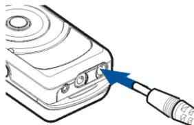
2. Connect the lead from the charger to the socket on the bottom of your phone. The charging time depends on the charger used. For example, charging a battery with the AC-1 charger takes up to 1 hour and 30 minutes while the phone is in the standby mode.
