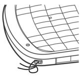
Thread the wrist strap as shown, and tighten it.
