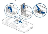
3 Insert the memory card, with the contact area facing down.
