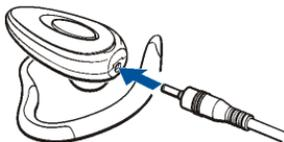
The headset is switched off and cannot be used during charging.
