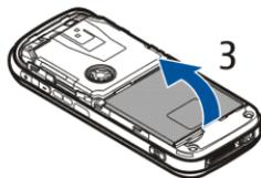
3. To release the SIM card holder, gently pull the locking clip of the card holder, and open it (4)
